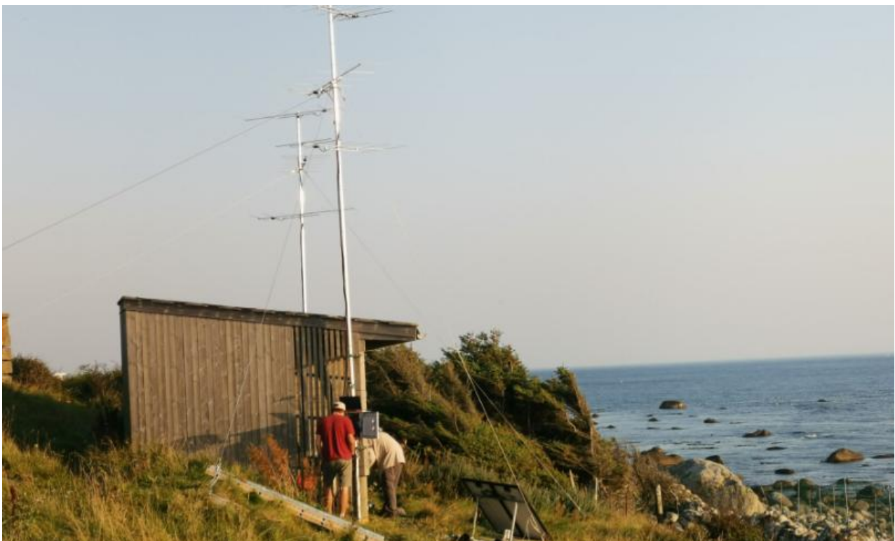
Two multidirectional MOTUS antennas are placed at the sea-watching hide, Lista Fyr.
